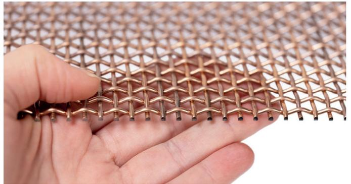
**Wire mesh:** Made of copper-plated steel
